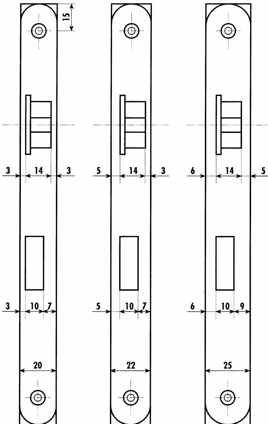
**ASAFSTAND****7 2****DISTANCE D'AXES****27A – 125A – 604 – 327 – 1604 - 328****RECHTS - LINKS****DROIT - GAUCHE**
